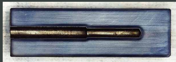
細穴/袋穴 真空浸炭品 Fine hole/blind hole vacuum carburized parts
