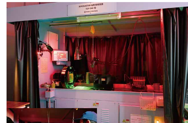
磁粉探傷検査設備 Magnetic Particle Inspection Equipment
