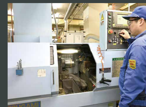
CNC内外複合研削盤 CNC internal and external combined grinding machine
