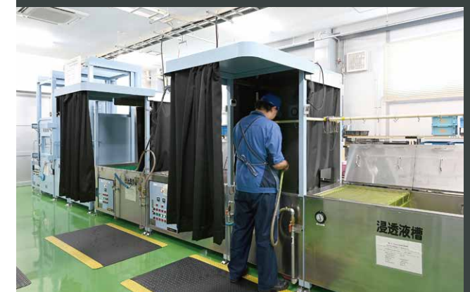
浸透探傷検査設備 Penetrant Inspection Equipment
